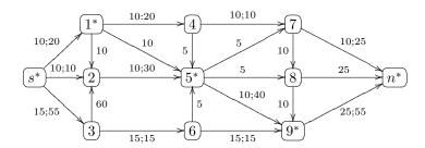
I put in three "easy" paths: sending 10 from s to 1 to 4 to 7 to n; sending 10 from s to 2 to 5 to 9 to n; sending 15 from s to 3 to 6 to 9 to n. I then applied the labeling rule to identify the path s to 1 to 5 to 9 to n. This path can carry ten units, so I add them.
