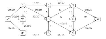
This is a solution. The minimum capacity cut has s, 2, and 3 in one set and the rest in the other set. The capacity of this cut is 65, which, of course, is equal to the maximum flow.
