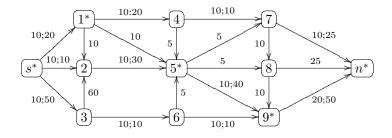
I put in three "easy" paths: sending 10 from s to 1 to 4 to 7 to n; sending 10 from s to 2 to 5 to 9 to n; sending 10 from s to 3 to 6 to 9 to n. I then applied the labeling rule to identify the path s to 1 to 5 to 9 to n. This path can carry ten units, so I add them.
