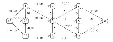
This is a solution. The minimum capacity cut has s, 2, and 3 in one set and the rest in the other set. The capacity of this cut is 60, which, of course, is equal to the maximum flow.
